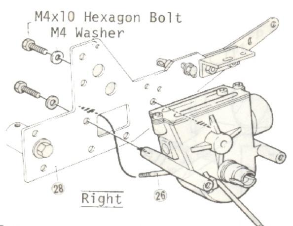
14 Insert gear box tension rod 26 through the square hole in the rear frame 28 and then install the gear box assembly onto rear frame 28.
