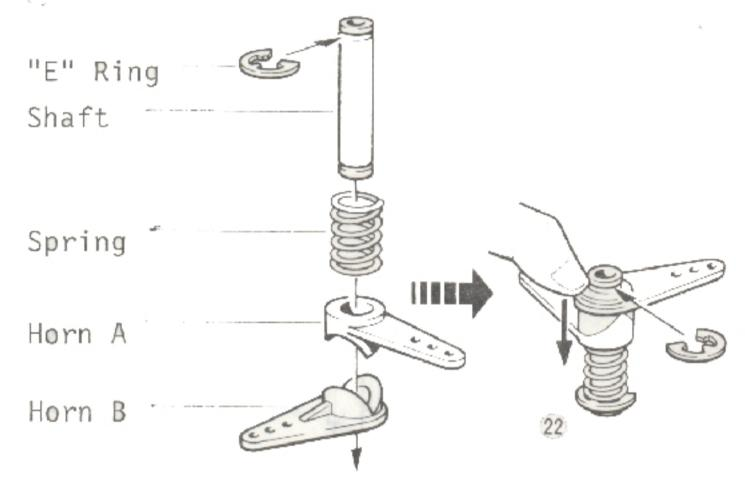
Servo saver 22 is already assembled. Use this illustration when disassembling and re-assembling.
