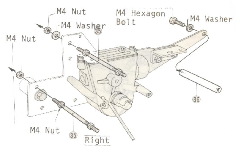
Screw on M4 nut onto stud bolt 35 as illustrated, and have stud bolt 35 temporarily attached to one side of the rear frame with M4 nut. Also, have rear bracket joint 36 installed as well.
