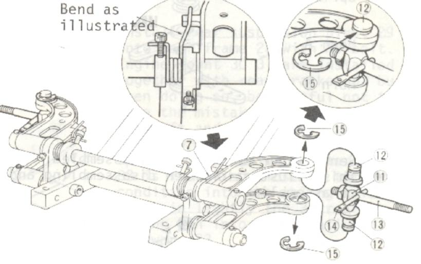
Insert into front suspension arm the already assembled parts (Key Nos. 1) 12 13 14 and then hold into place with "E" ring 15. Next, set the front spring 7 into place as illustrated.
