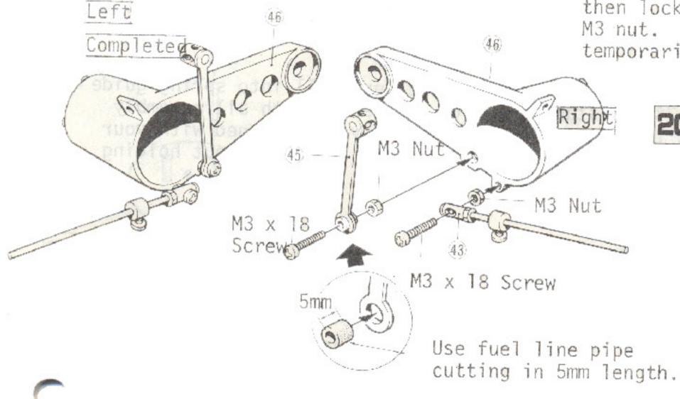
Install stabilizer link 45 and spring guide end 43 onto rear suspension arm 46 as illustrated. When installing, set so that there will be no excess play on the left or right side and also make it so that the movement is free then lock with M3 nut. For people installing rear damper (option), see page 12 illustration 49.
