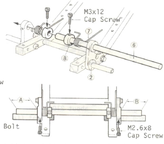
In order not to make a mistake on the right and left front spring, arm axle B 6 is set into place with M2.6 cap screw onto arm holder(2) as illustrated. But it is stabilized making the length of A . B in the same length as shown in illustration below.
