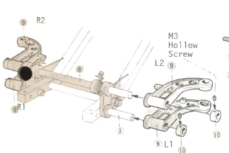
As L1, L2, R1, R2 are stamped on the each front suspension arm 9, using illustration as reference, insert arm axle A 3 and B 6 and then is installed with suspension side stopper 10 but when doing so, set it so the there will be no excess play to the right and left on the suspension arm and have it so it will move up and down freely.
