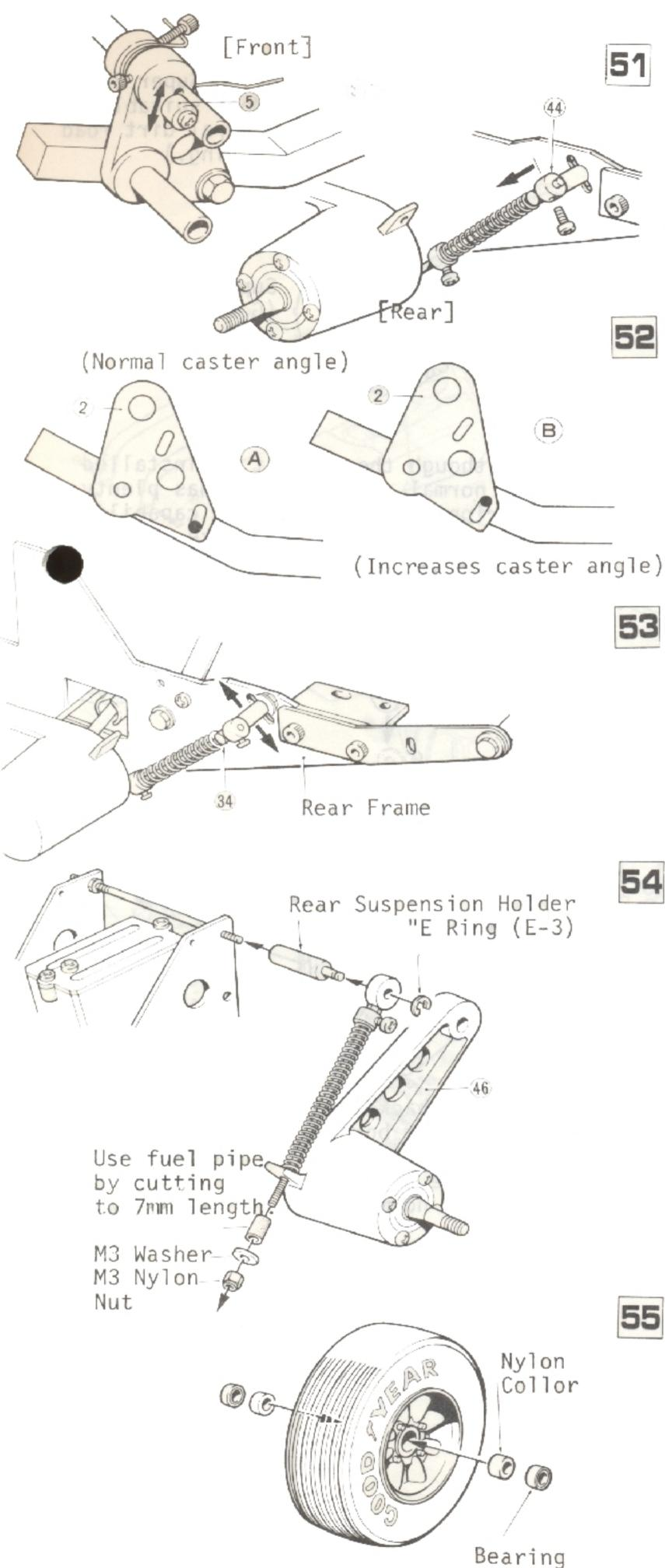
The vehicle height is adjusted by moving the 5 suspension stopper to the top of the arrow making the front low and vise versa making it high. For the rear, by moving the 44 3ø stopper down in will make it go down and high for vise versa, set the height depending on the road condition.
