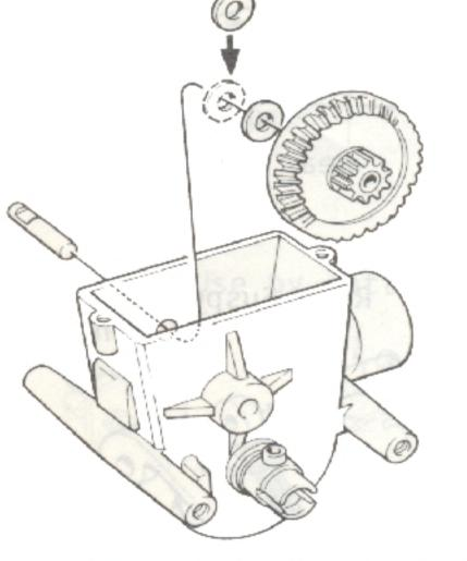
When the back-lash on the bevel gear in the gear box has become large, by insterting a 5¢ washer included in the spare screw bag, maintain a constant normal mesh of the gears.
