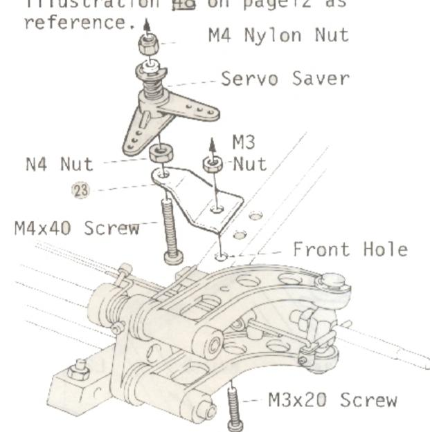
Install servo installation hardware 23 onto main frame, stabilize firmly with M4 nut the M4x40 screw onto hardware 23, insert M4 screw through the servo saver, and is set into place with M4 nylon nut but make sure that the nylon nut is not tightened too much in order to keep a light movement to the left and right.
