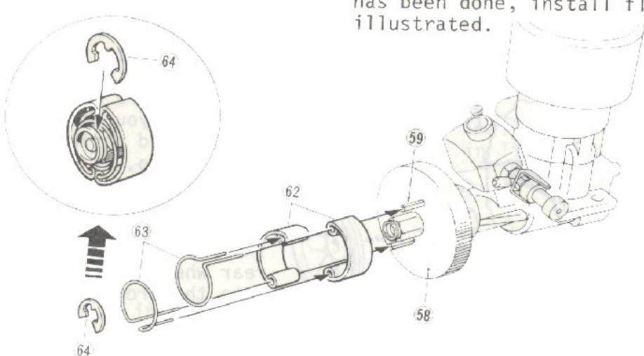
Insert clutch shoe 62 into clutch pin 59, as illustrated, insert the longer side of the clutch spring 63 into clutch pin 59 hole and the shorter side into clutch shoe 62 hole. And finally fit into the groove of the pilot nut the pilot "E" ring 64 and make it so that & the spring will not come off.
