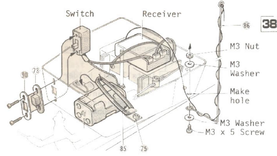
When installing switch as illustrated. Stabilize the switch into place using 73 switch rubber boots and 90 switch plate. Stabilize battery onto 75 battery holder hardware with 85 rubber band. The receiver is placed on top of the servo. Install 86 antenna guide onto the mechanism box as illustrated.
