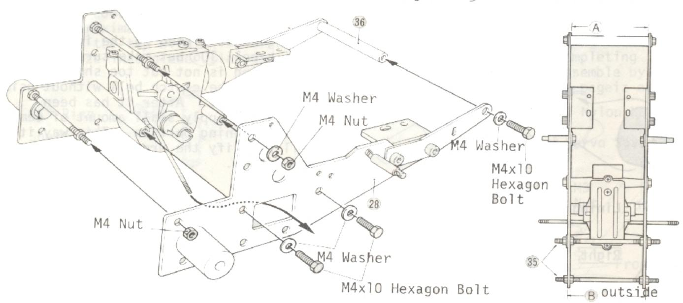
The other side rear frame 28 is installed as illustrated but tighten by adjusting the M4 nut on the stud bolt 35 so that the A B will be parallel as illustrated.
