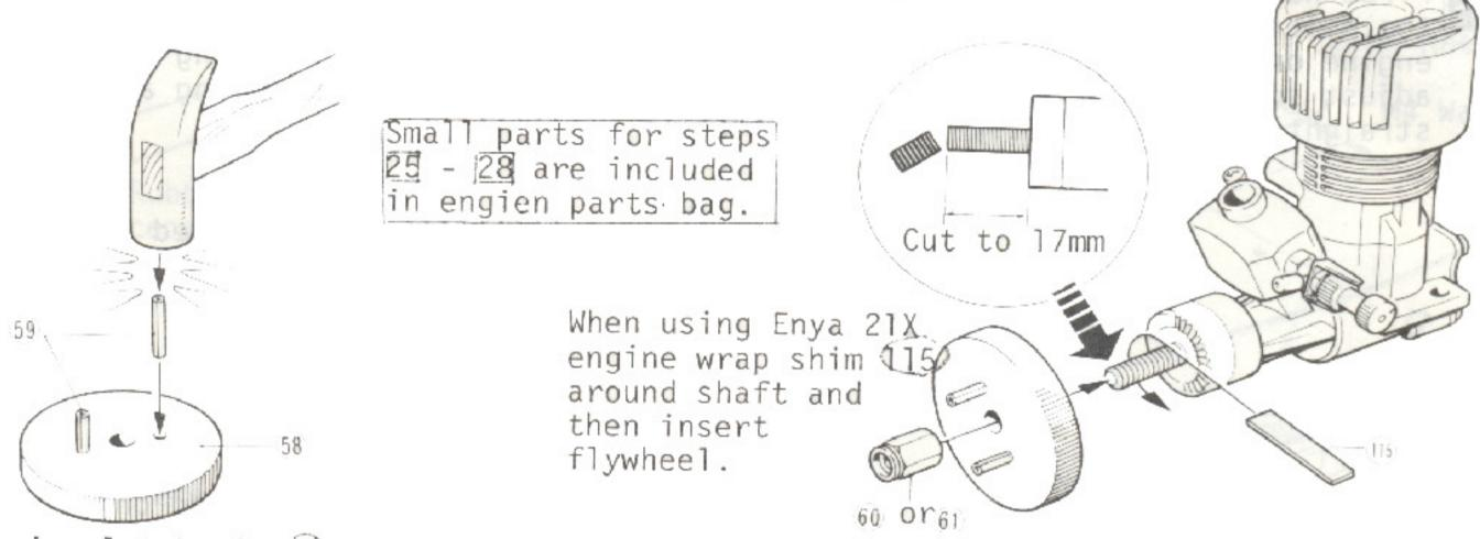
25 Top in clutch pin 69 into Flywheel 58.
