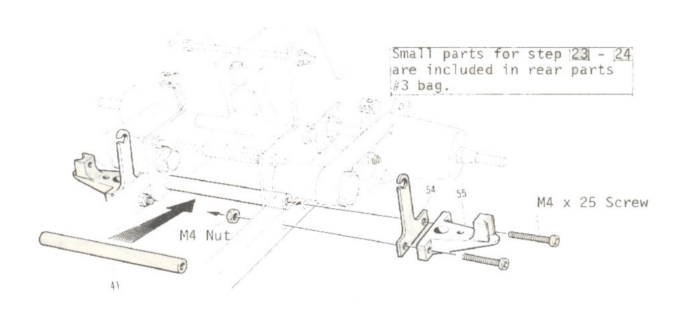
23 Set the joint collar 41 into place onto the inner side of the chassis. Stabilizer installation hardware 54 and side member 55 are installed.
