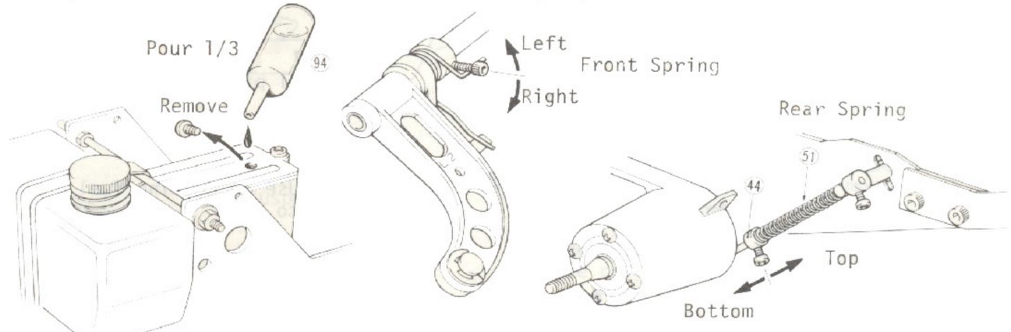
Remove the M4 screw on the lid of the gear box and through this hole, fill with 94 oil (5cc) which is included in kit.
