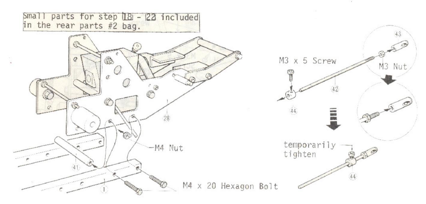
Install rear frame 28 onto main frame as illustrated.
