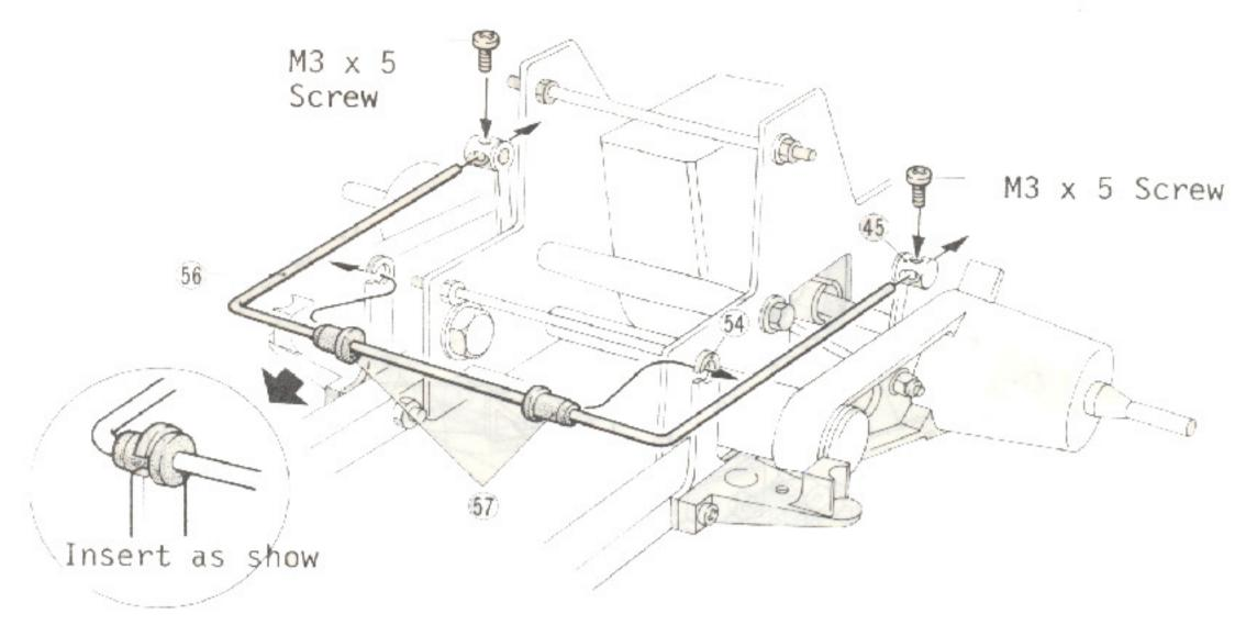
Insert rubber bushing 57 into stabilizer 56 as illustrated. As the stabilizer 56 is being inserted into stabilizer link 45, fit the rubber bushing 57 into 54 from the inner side and stabilize onto stabilizer link 45 with M3 x 5 screw.
