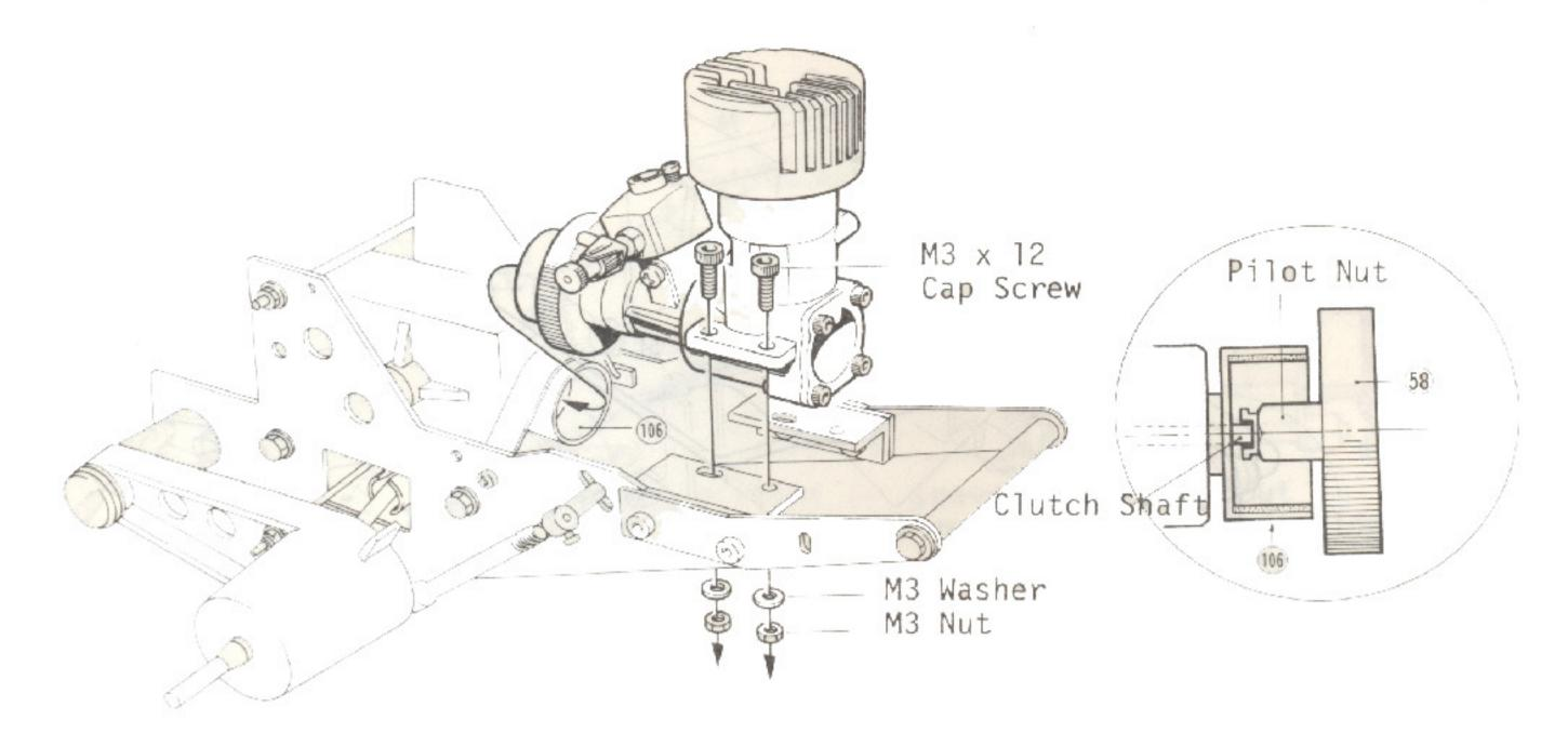
First have the bolt holding the engine mount loosened, align the center hole of the pilot nut and the clutch shaft of the clutch bell 106 and then install the engine onto the engine mount. At this time, as each bolts are being tightened adjust so that the engine and the frame will become parallel looking at it from straight top and directly fram the side.
