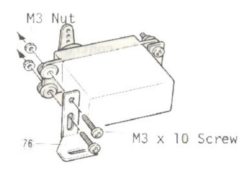
Servo bracket 76 is installed onto the steering as well as to the throttle control servos.
