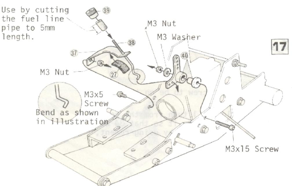
Cement lining 27 onto brake shoe 37 then install brake and "L" crank 40 as illustrated. Screw in brake adjuster 39 into brake rod 88.
