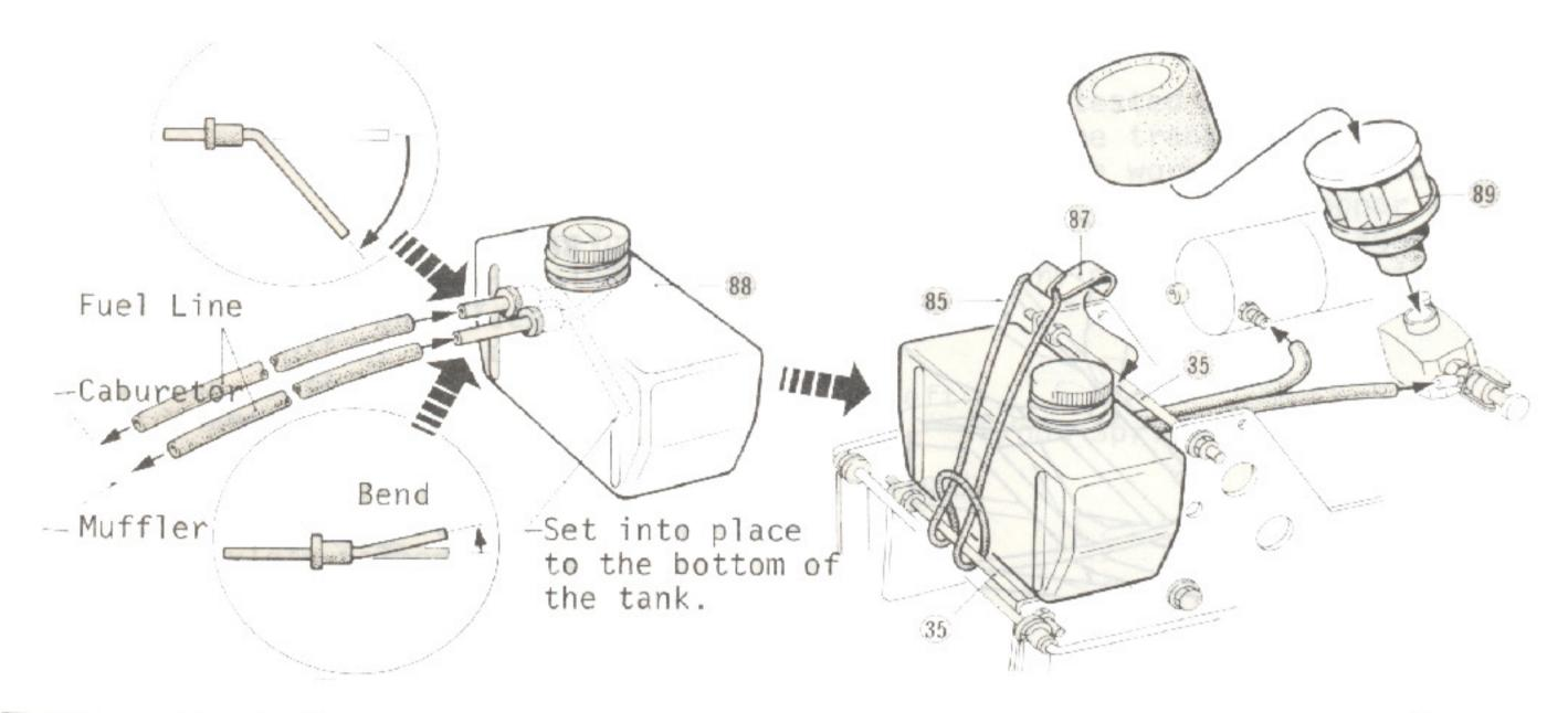
Assemble fuel tank as illustrated. For installation, hook rubber band 85 onto stud bolt 35 and stabilize into place by hooking the 87 tank installation hardware onto the upper stud bolt 35. Install the 89 air filter assembled in step 32 onto the carburetor.
