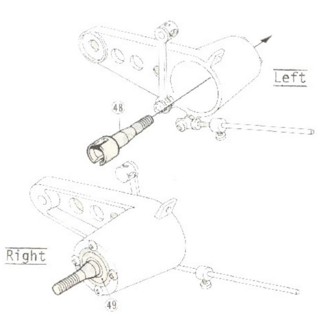
Rear wheel shaft 48 is inserted into rear shaft bearing 49.
