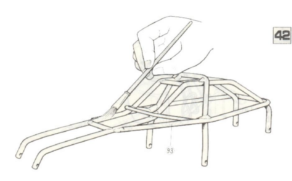
Body 93 is painted but before painting, check to see if the chassis and body installation holes are in line and in case it is out of line, adjust with plier or other comparable tool. Also, before painting, wash away dirt and oil with neutral liquid soap. Paint to be used should be for vinly type and fuel proof (engine color, etc.).
