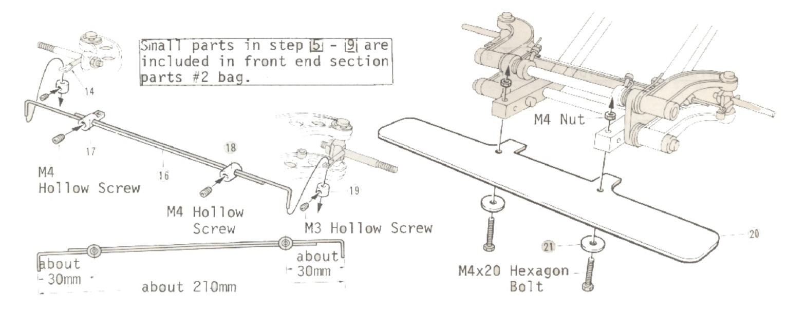
Insert through tap a 17 and top B 18 the tie rod 16, make the total length of the tie rod about 210 mm long, position the tap approximately 30 mm from the end, install the tap with M4 hollow screw and stabilize into place using tie rod stopper 19.
